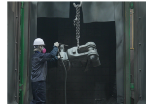
Shot Blasting Shooting(Surface)
